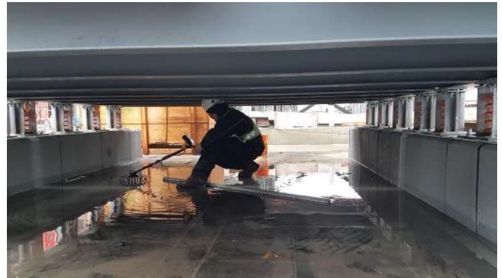
The flexible design of the Digiscan 360 allows scanning of difficult to access areas where damages would otherwise go unnoticed
