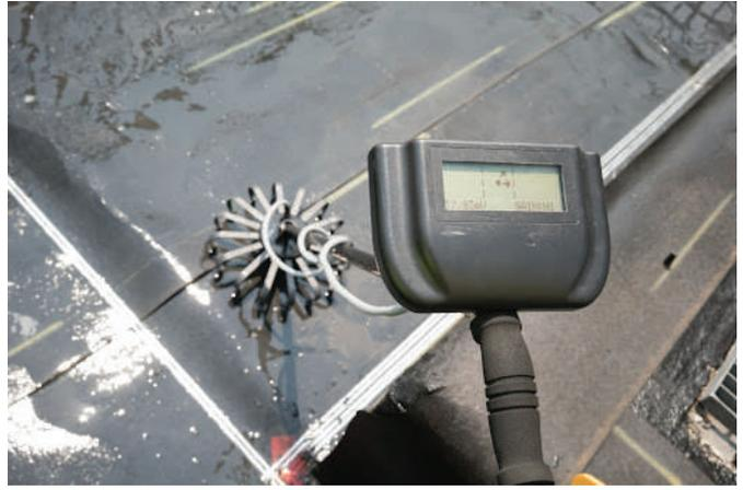
Leaks and penetrations are found on a roof membrane after the first scan
