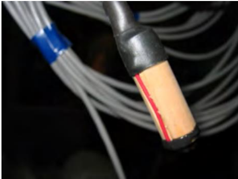
Image 8: Embedded moisture sensor with wood plug (SMT).
