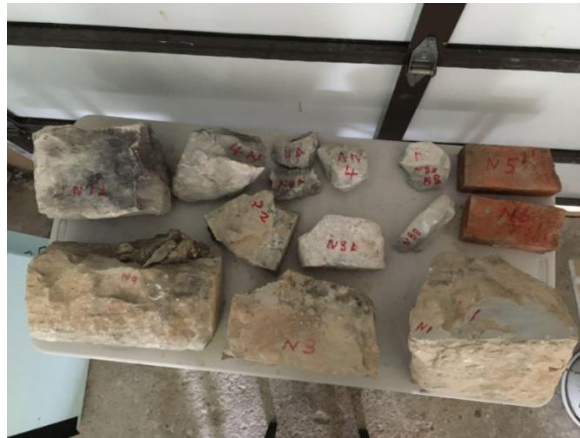
Image 6: Masonry samples collected from exploratory openings to be tested to obtain physical properties (Building Enclosure Labs Inc., 2021).
