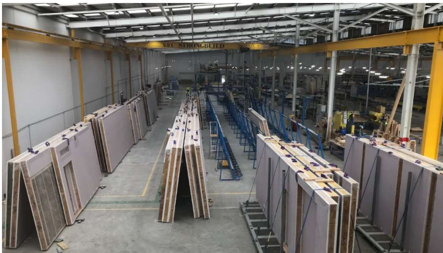
Figure 3: Finished wall frames waiting for delivery to site, Image Credit: Strongbuild
