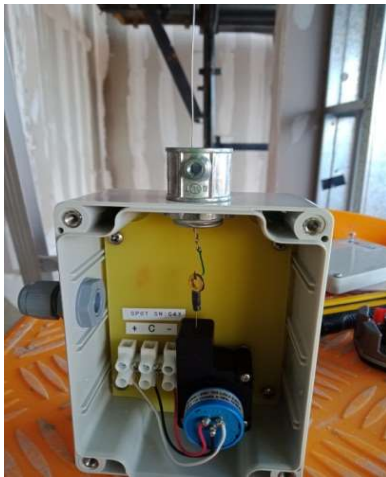
Figure 14: Connection of a fishing hook and the displacement sensor, Image Credit: TDA
