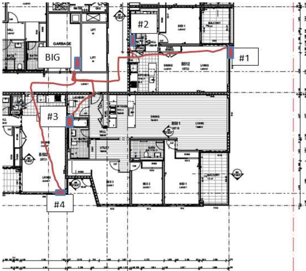
Figure 24: Position of wires connecting sensors and A3's, Image credit: Strongbuild
